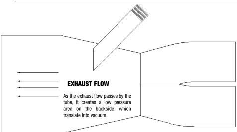
**Note:** Your Edelbrock Victor Series Race Headers include stainless steel evacuation tubes, 02 sensor bungs and collector mounting tabs to be installed, if needed. Collector mounting tabs should be installed after primary tube tuning has been completed. Evacuation tubes can be positioned on the collector where desired for best fit and hose routing. See the above diagram for recommended installation.
